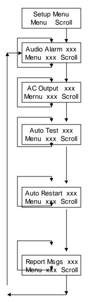
**Note:** At any step in the "Setup" menu, pressing the "MENU" selection will move you to the "Config" menu.
